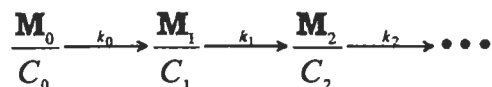
Fig. 1 Schematic model of deteriorating cascade by materials started from M_0 , and followed by M_1 , M_2 , \dots . Concentrations are described by C_0(t) , C_1(t) , C_2(t) , \dots .
